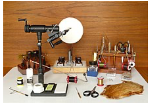
Various tools enable and optimize fly tying. Skip Morris, a professional fly tyer, lists the essential tools as being a vise to hold the hook of the fly to be tied, bobbin holders , hackle pliers , hackle gauges , work lights and magnifying glass to better see the fly as it is tied, hair stackers , scissors and tweezers . Other optional tools are pliers , toothpicks , bodkins , [19] dubbing twisters , blenders , floss bobbin holders , whip finishers , wing burners and
